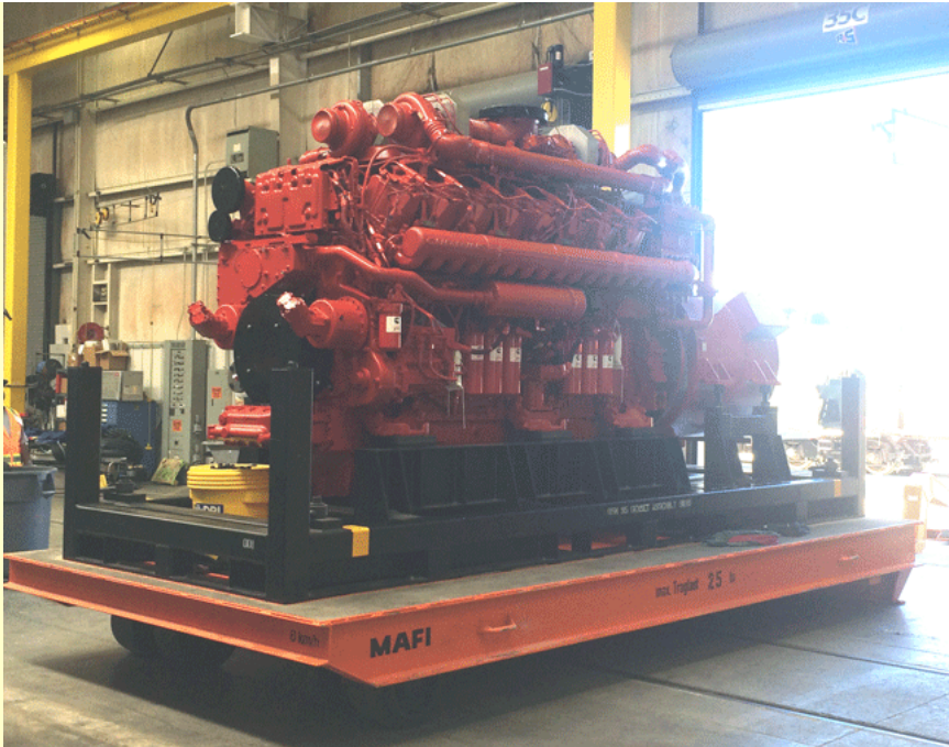
Cummins 4,400 hp diesel engine (Photo by G. Huckaby)
