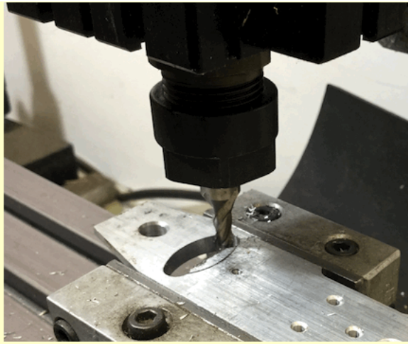
Figure 3 - Reaming out the opening for the center truck power pickups.
