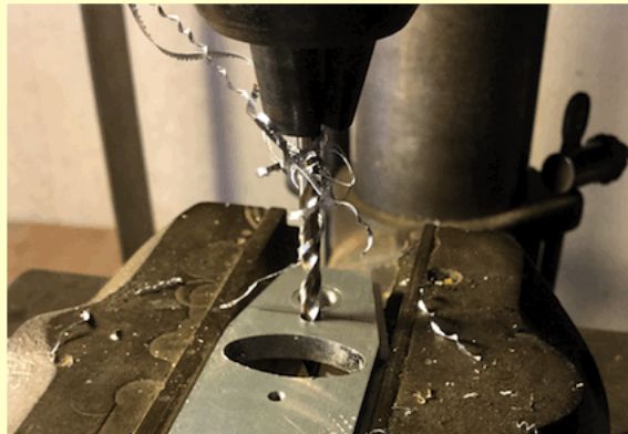
Figure 5 - Drilling hole for center pivot.
